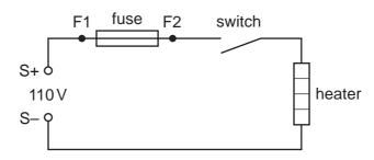
Owing to a fault in the system, power is not supplied to the heater. A technician diagnoses the fault using a voltmeter.
